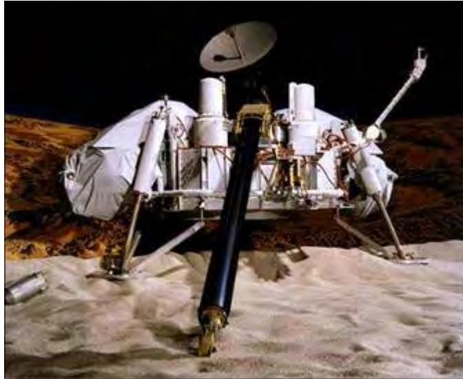
Figure 21: One of the Viking landers with its mechanical arm deployed (Credit photo: NASA/JPL).
